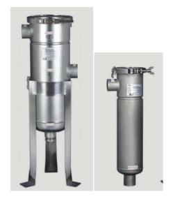
MEY's MEBH single bag filter stainless steel housing with a economical design, the V-clamp band top closure convenient for quick and easy to opening the top cover and replacement the filter bags. .As standard, the MEBH series is provided with heady duty adjustable mounting bracket support legs and SS filter basket supplied to support for the filter bag.Suitable for the general commercial and industrial applications liquid applications
